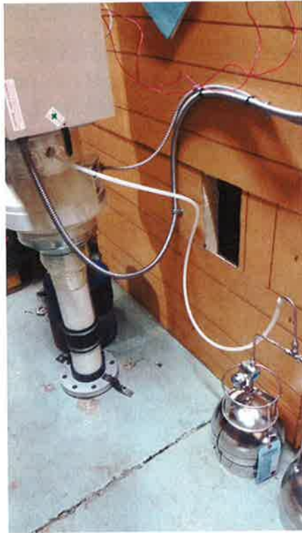
Photograph 1: View of soil vapor collection point installed in the 4-inch diameter PVC piping connecting the fan to the electric heater. Tubing connects the sample port to the 6-Liter Summa canisters in the bottom right of the photograph.
