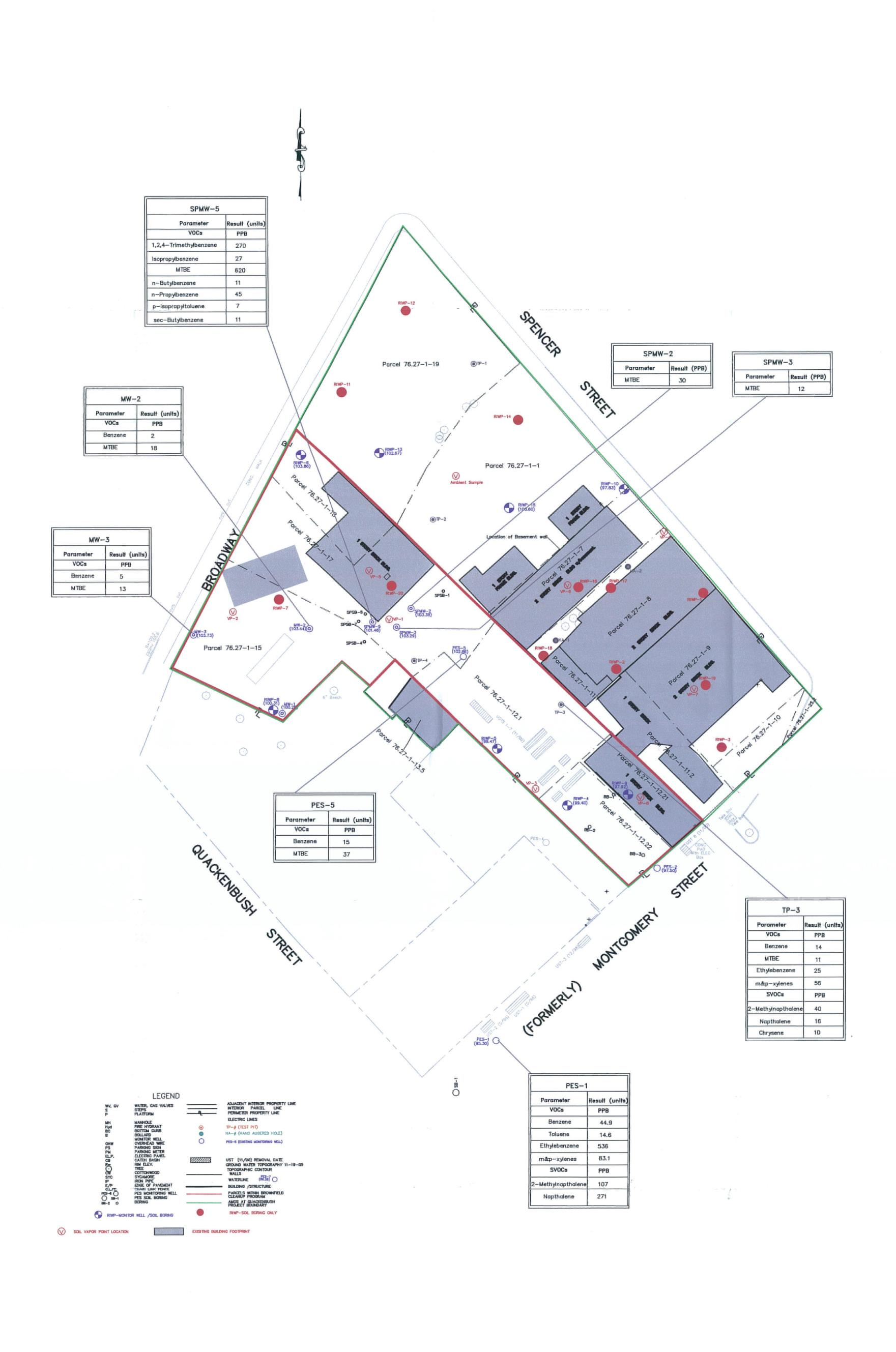
NOTES: 1. ALL ELEVATIONS ARE REFERENCED TO AN ASSUMED DATUM. SUBTRACT 79.17 FT, TO CONVERT TO THE NATIONAL GEODETIC VERTICAL DATUM (N.G.V.D.)
