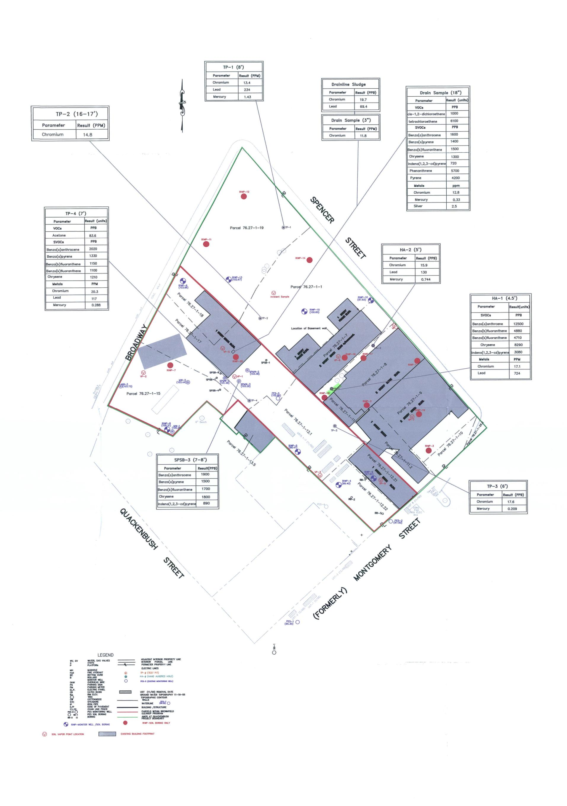
NOTES: 1. ALL ELEVATIONS ARE REFERENCED TO AN ASSUMED DATUM. SUBTRACT 79.17 FT. TO CONVERT TO THE NATIONAL GEODETIC VERTICAL DATUM (N.G.V.D.)
