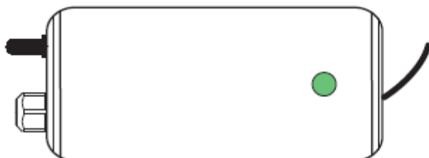
Green LED indicates UV lamp "ON".
