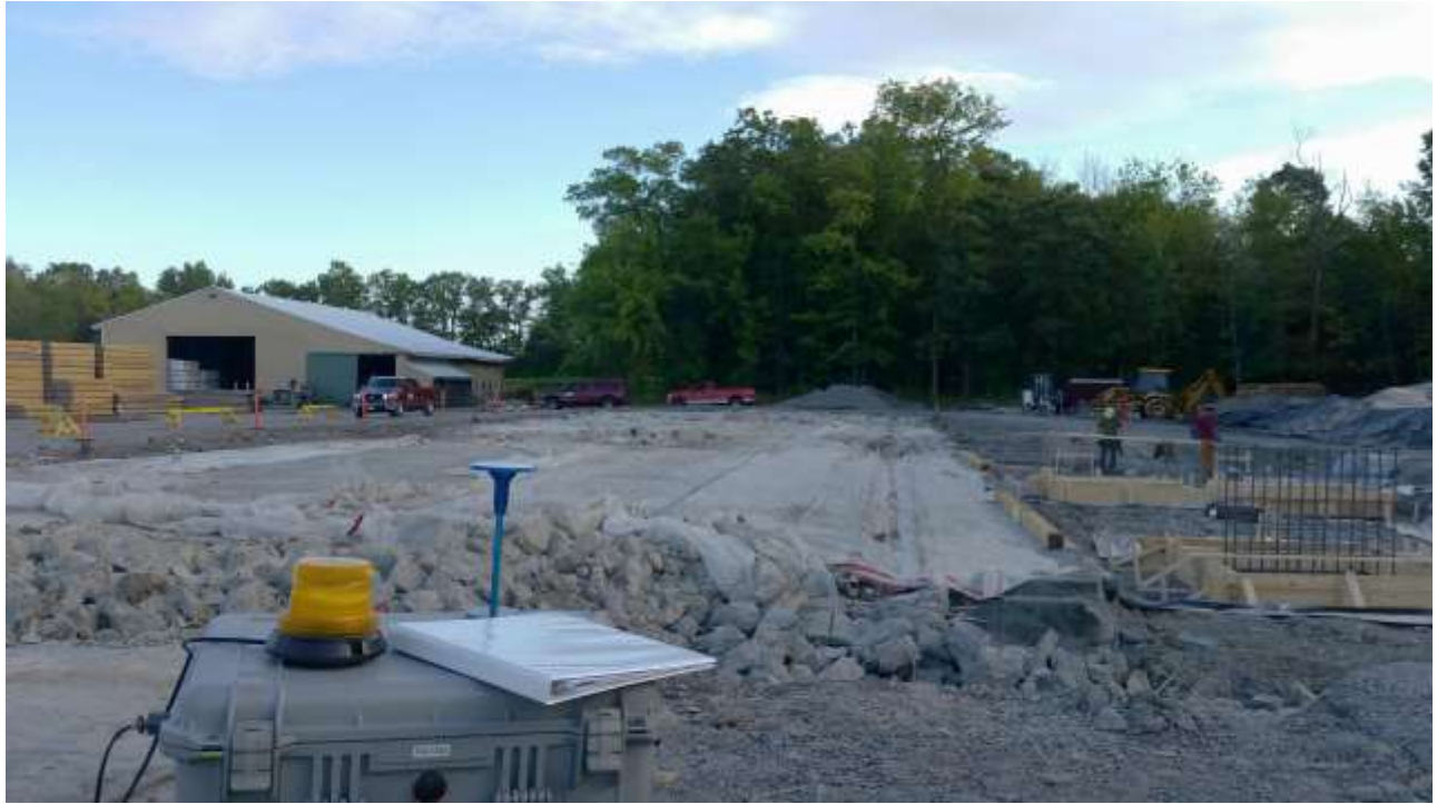
Photograph 5: Community Air Monitoring and Worker Breathing Zone Monitoring were conducted with three (3) DustTrak II Aerosol Monitors with audible and visual alarms. Breathing zone monitor shown.
