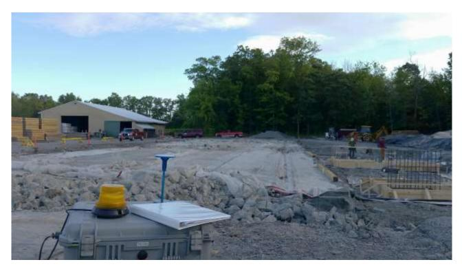
Photograph 5: Community Air Monitoring and Worker Breathing Zone Monitoring were conducted with three(3) DustTrak II Aerosol Monitors with audible and visual alarms. Breathing zone monitor shown.
