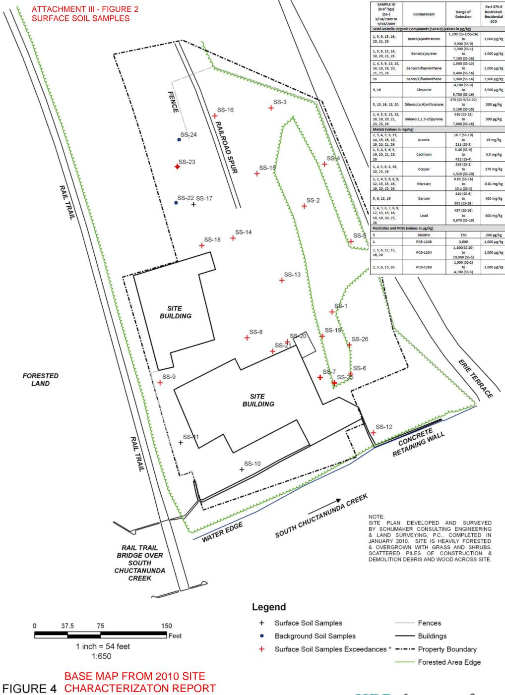
FIGURE 4 CHARACTERIZATON REPORT SURFACE SOIL SAMPLES NATHAN'S WASTE & PAPER STOCK ERIE TERRACE AMSTERDAM, NEW YORK HRP # NEW9506.P2 SCALE 1:650
