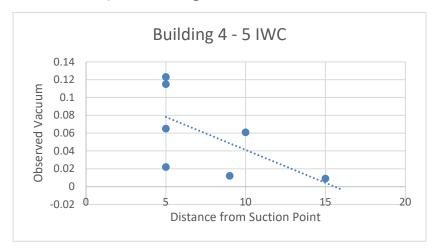
The maximum ROI was determined to be approximately 16 feet at 5 IWC at the suction point. This ROI was determined solely from the southwest measuring points due to the interference of the foundation as measuring points 4NW10, 4NE15, 4SE10 are located on the outside of the foundation barrier.
