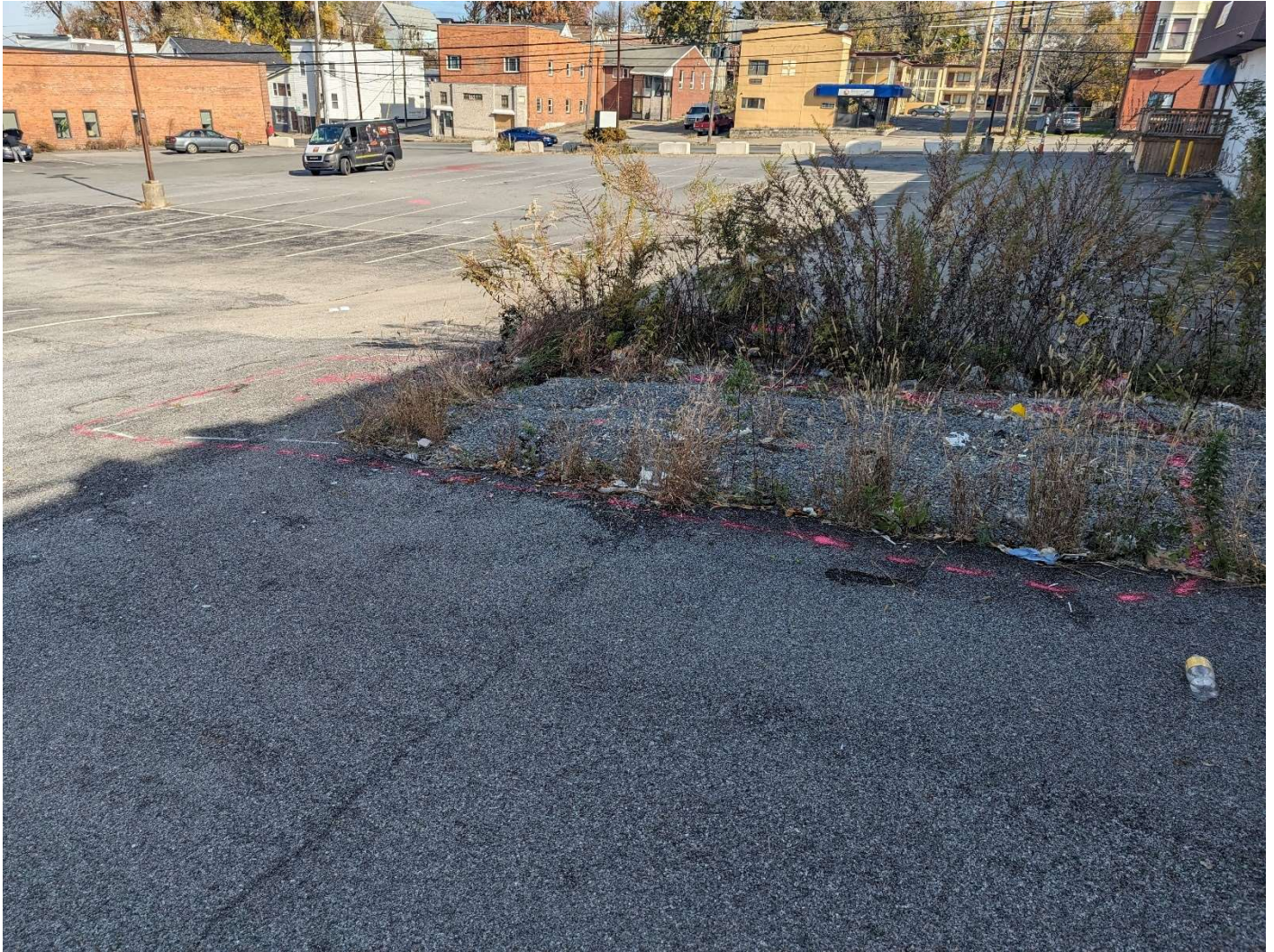
Second suspected UST location with an approximate depth of 2.5 – 5 feet. (Sloped ground resulted in the tank being at greater depth at the top of the hill)
