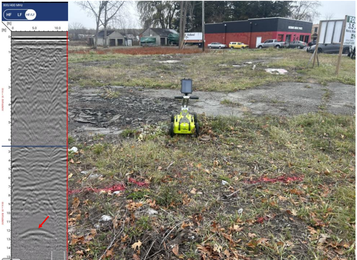
GPR Reaction Showing a Storm Drain:
