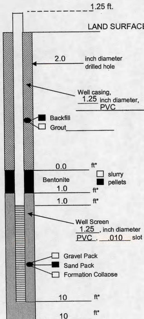
Project Number 06.6448Project Name Old Champlain Mill Phase II ESAWell No. MW-10 Boring No. GP-10Town/City Village of WhitehallCounty Washington State New YorkInstallation Date(s) 11/16/06Drilling Contractor ADT, Inc.Drilling Method Van Mounted GeoprobeWater Depth From Top of Riser 4.12 ft 11/17/06
