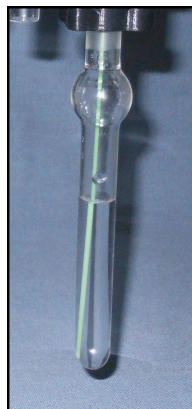
Figure 8.1-4: Look for Bubbles in the sparge bottle.
