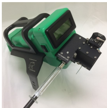
Figure 8.1-2: Pushing water from the plumbing.
