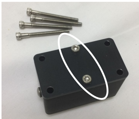
Figure 7.3-4: Two Center Screws hold the lid on the scrubber block.
