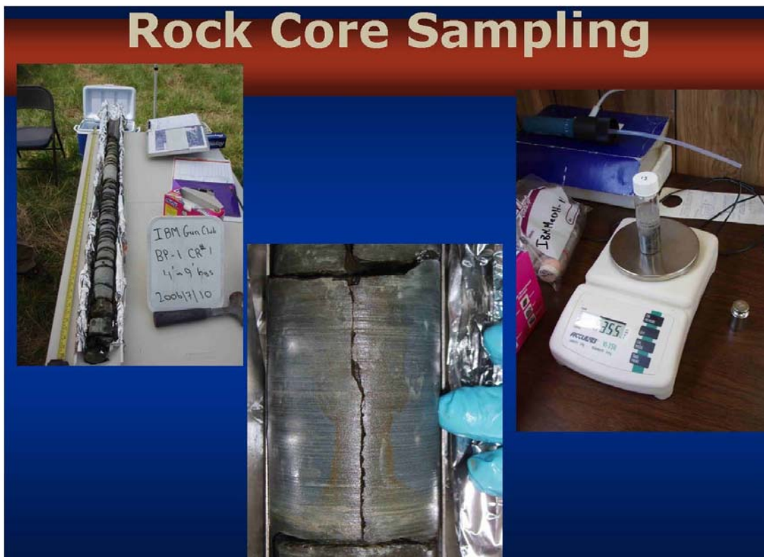
Exhibit 5.2 – Photos of Rock Core Sampling- depicting counterclockwise from upper left, photo documentation of a 4-foot core run, a close-up of a segment of core with a stained vertical fracture and oily sheen, and weighing crushed rock sample in vials of methanol.
