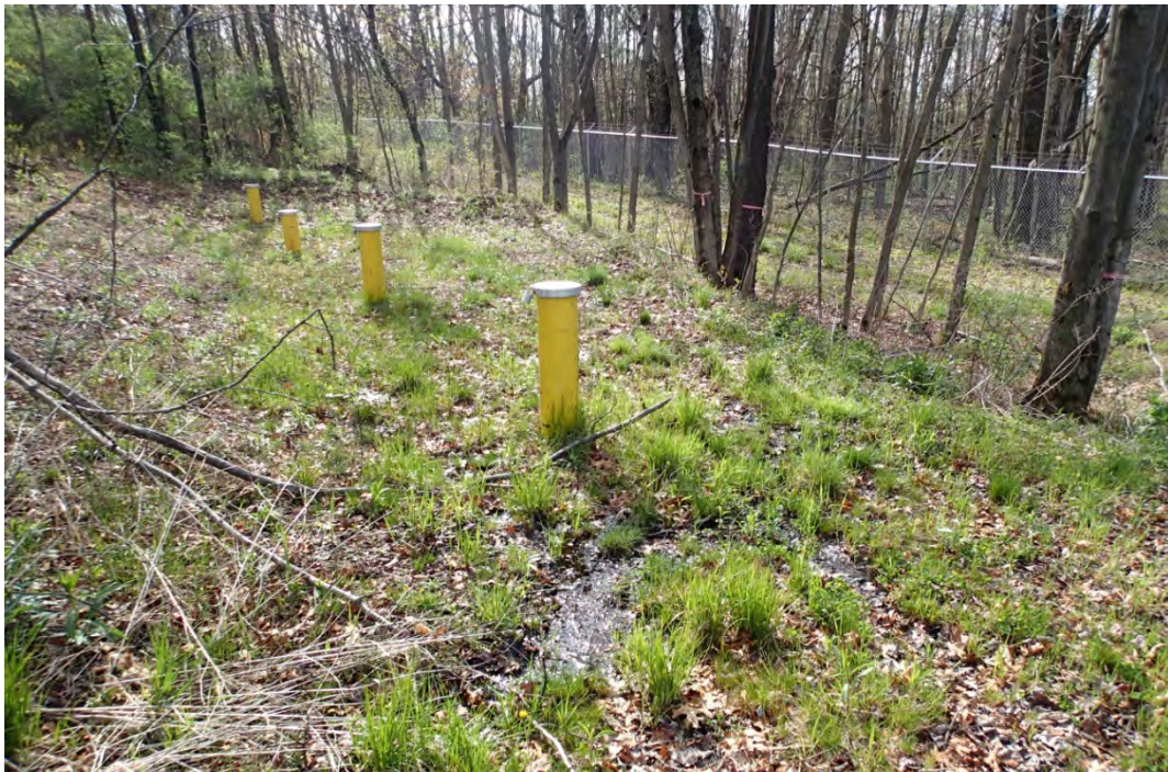
Photo 10: Flowing seep present on the eastern edge of seep fill area, looking at injection borehole B-10.
