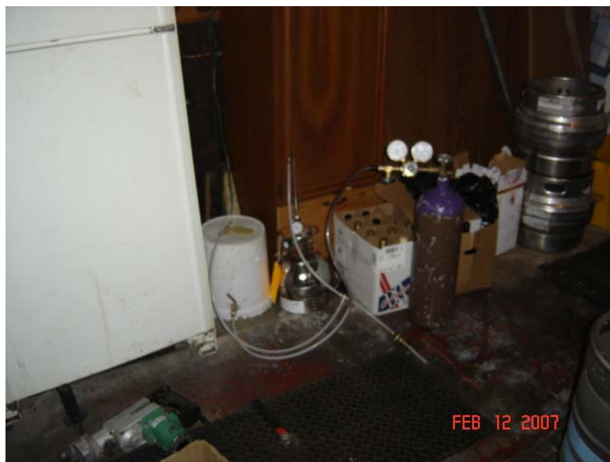
Photo 3 Sampling Location SS-1 Helium Added to the Trap
