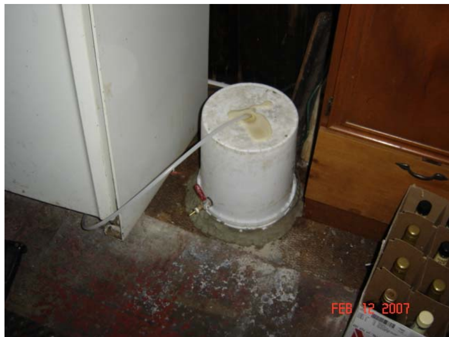
Photo 2 Sampling Location SS-1 Helium Trap Setup
