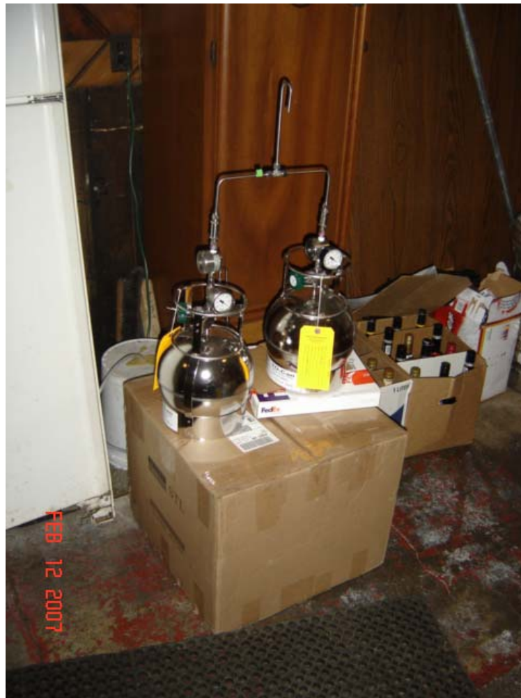
Photo 5 Sampling Location IA-1 “T” Connection Used to Collect a Blind Duplicate Sample
