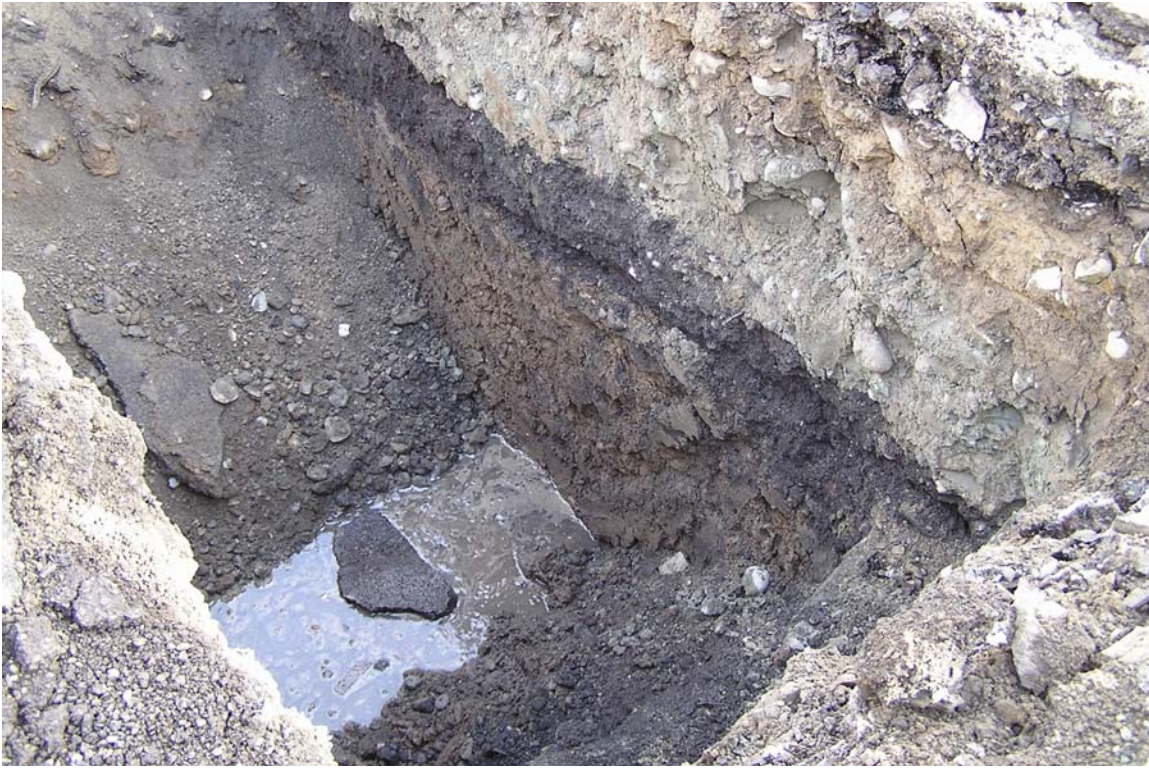
Photograph 3: View of sheen on water in a test pit excavated at Area H on the Gannett Parcel.
