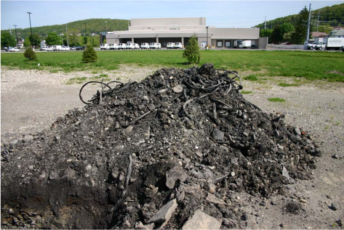
Photograph 1: View of fill material encountered at Test Pit 1
