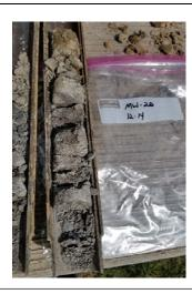
OU2 – Overburden Basal Till to Weathered Bedrock Transition Sample
