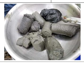
OU3 – Former Canal Typical Sediment Core Recovery
