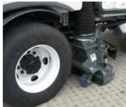
Routine, air-vacuum sweeping in the early spring and fall is the best approach for porous pavement maintenance (Photo source: Toronto and Region Conservation)
