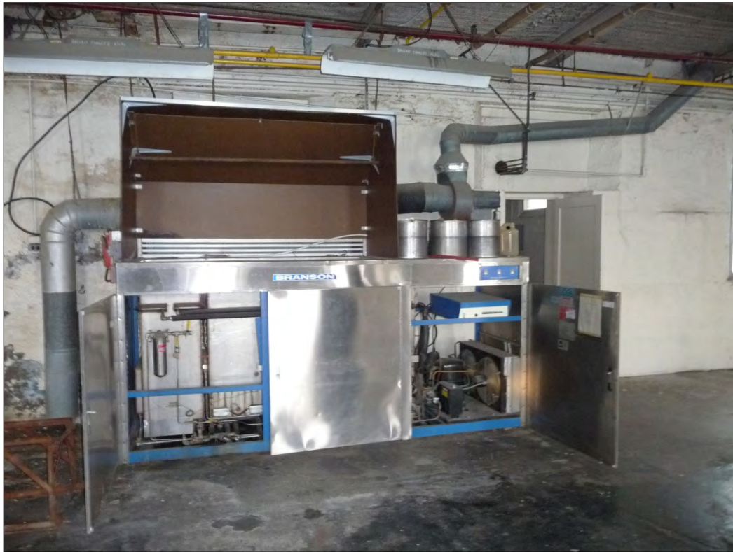
TCE vapor degreaser with vent to outside.
