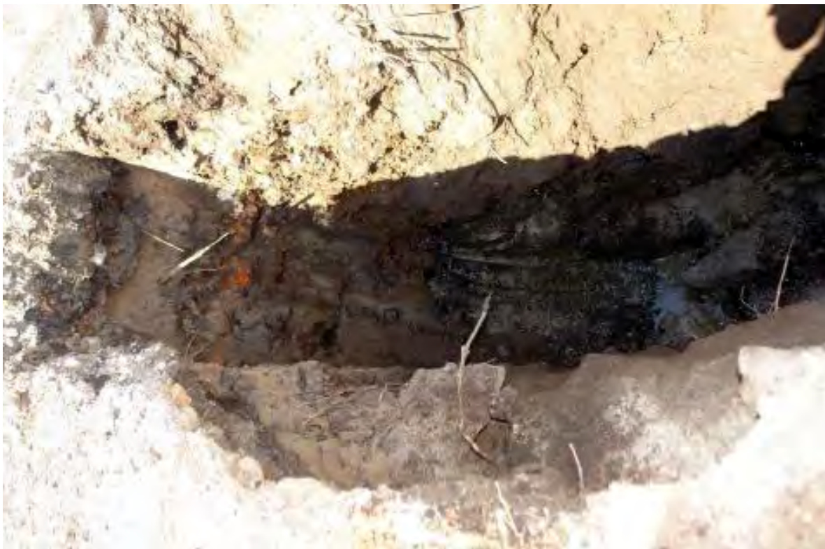
Slag and fill material in parking lot (former disposal area) behind manufacturing building.
