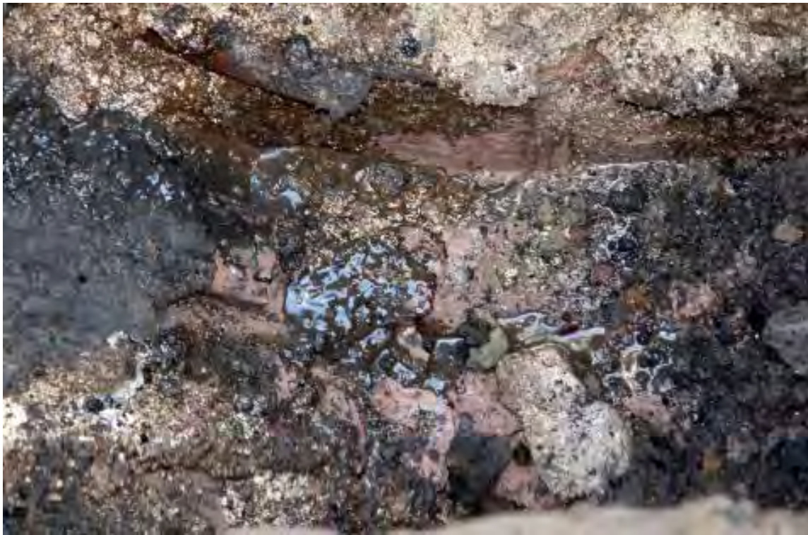
Buried slag in excavation behind former manufacturing area of site, northeast site of building
