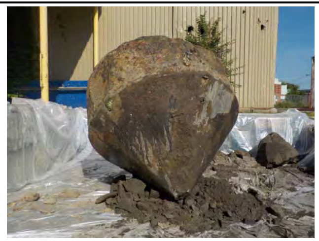
Photograph 28. Second tank removed. Holes and thin steel noted at the bottom of the tank.
