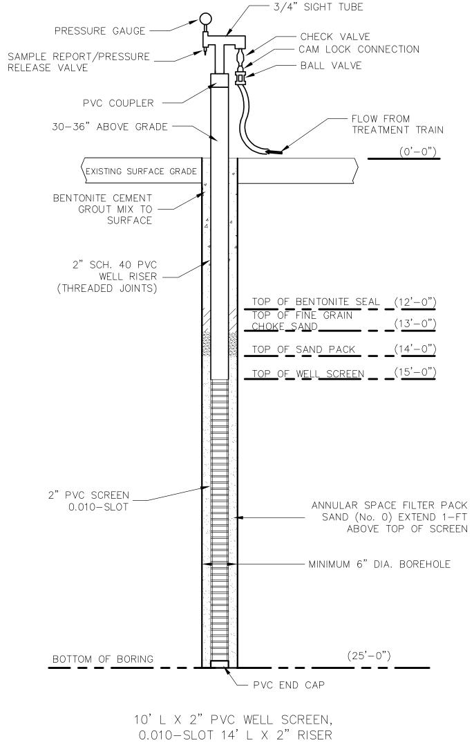
2 TYPICAL INJECTION WELL DETAIL NOT TO SCALE
