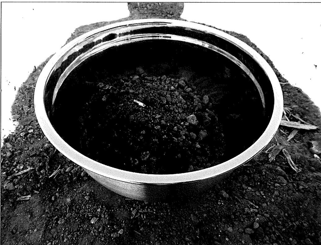
**PHOTO 8:** Example composite of individual grab samples from a fill area section
