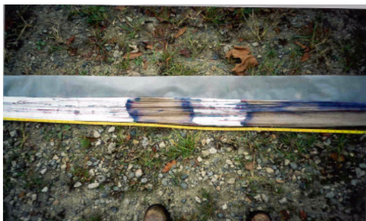
Fig. 4.1.2. Stains from TCE in fractures. The normally white inside surface of the NAPL cover shows where TCE has contacted the cover in a 3 inch core-hole. The core from this borehole showed no NAPL in the fractures probably due to flushing by drilling fluid.
