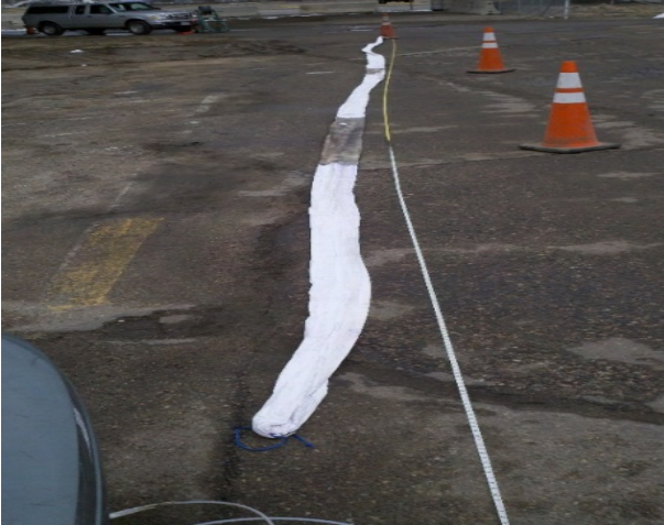
Fig. 4.1.3 Stains on the inside surface of a NAPL FLUTE showing the location of the DNAPL. Tape measure on the right provides depth BGS.
