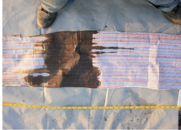
Fig. 4.1.4. Coal tar stains at a fracture observed on the NAPL FLUTE cover in a 4 inch borehole.
