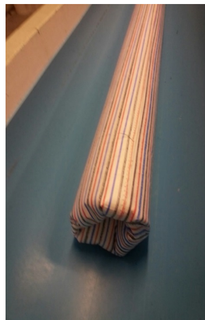
Fig. 4.1.1. Dye striped exterior of a NAPL FLUTE cover as mounted on the exterior of an everting blank carrier liner.
