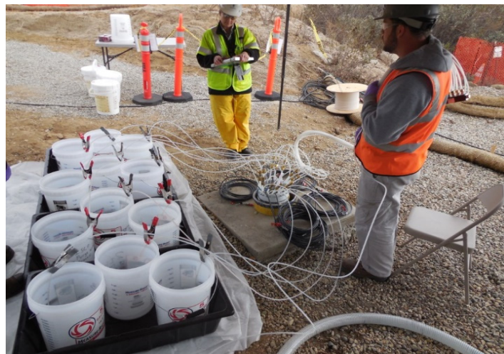
Fig. 7.2.2. Simultaneous purge of 12 ports with monitoring of purge volume from each port.
