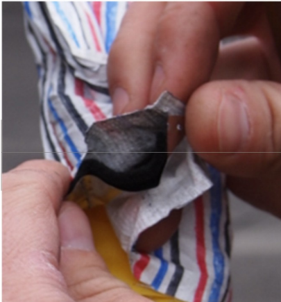
Fig. 2. The carbon felt between the cover and the diffusion barrier
