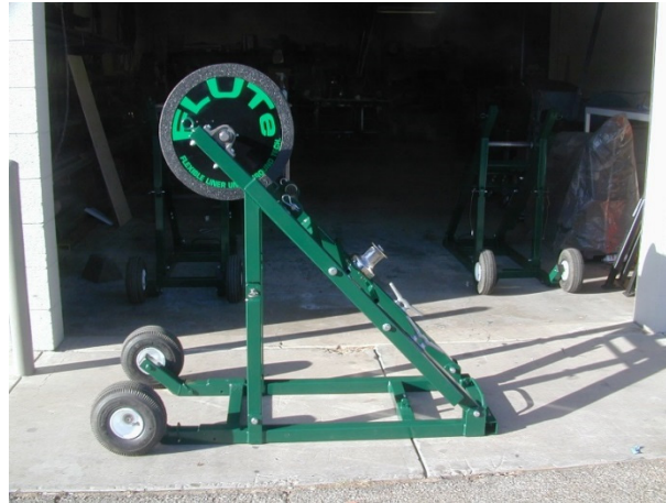
Fig. 3.2.1. Photo of the Green Machine showing the wellhead roller and capstan used to winch the liner from the borehole. The machine folds to a relatively flat profile for shipment.
