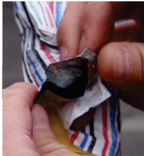
Fig. 4.2.2. Photo of FACT showing the dye striped NAPL FLUTE cover, the black carbon felt, and the silver diffusion barrier.
