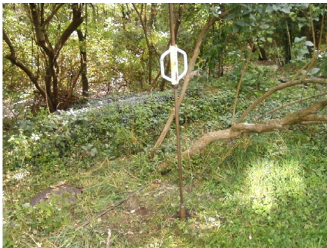
Geoprobe® Slide Hammer to install SV-19
