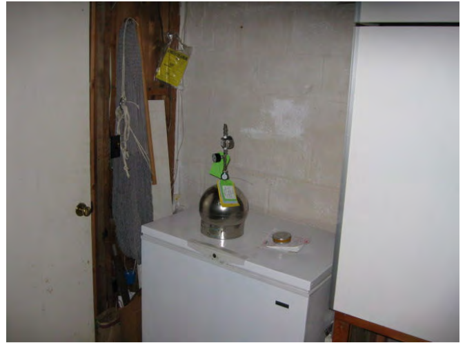
Basement Air and Radon Samples – Structure 39
