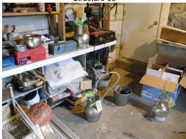
Structure 37 – Basement Air and Sub-Slab Vapor
