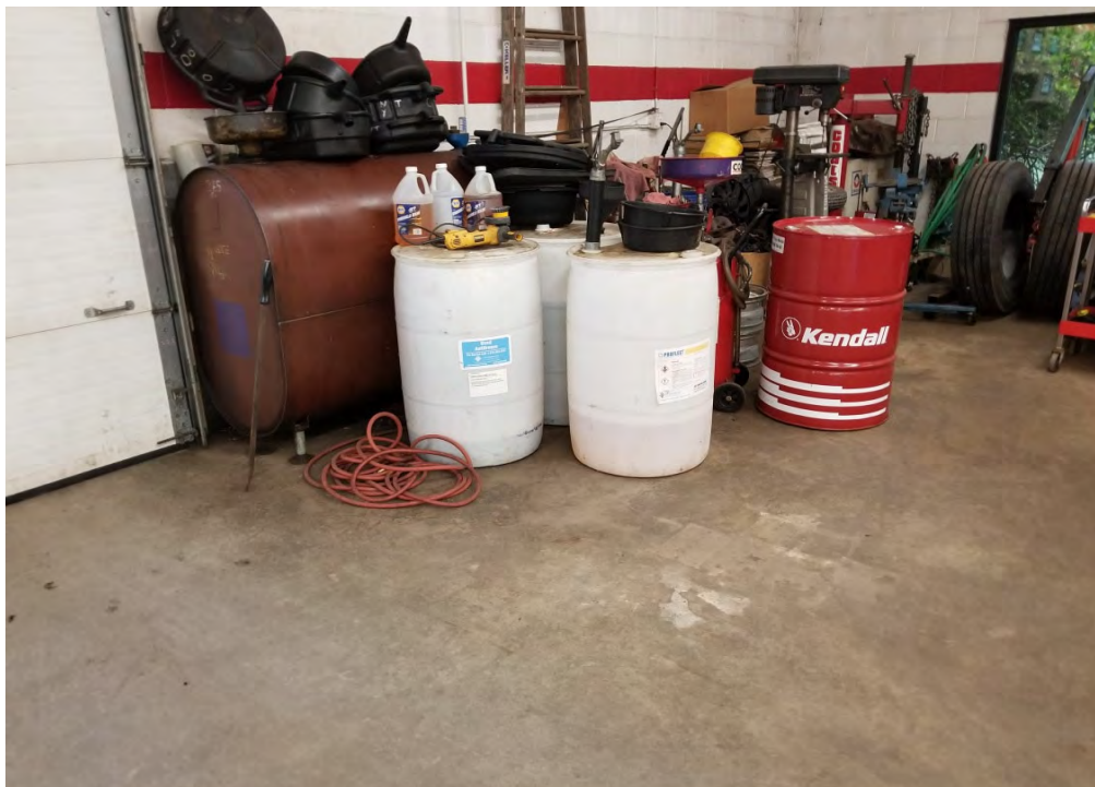
4. Southwest view - View of the 55-gallon drums for used antifreeze, a 265-gallon waste-oil AST, and a 55-gallon drum of new oil located on the southwest interior of the on-Site structure.
