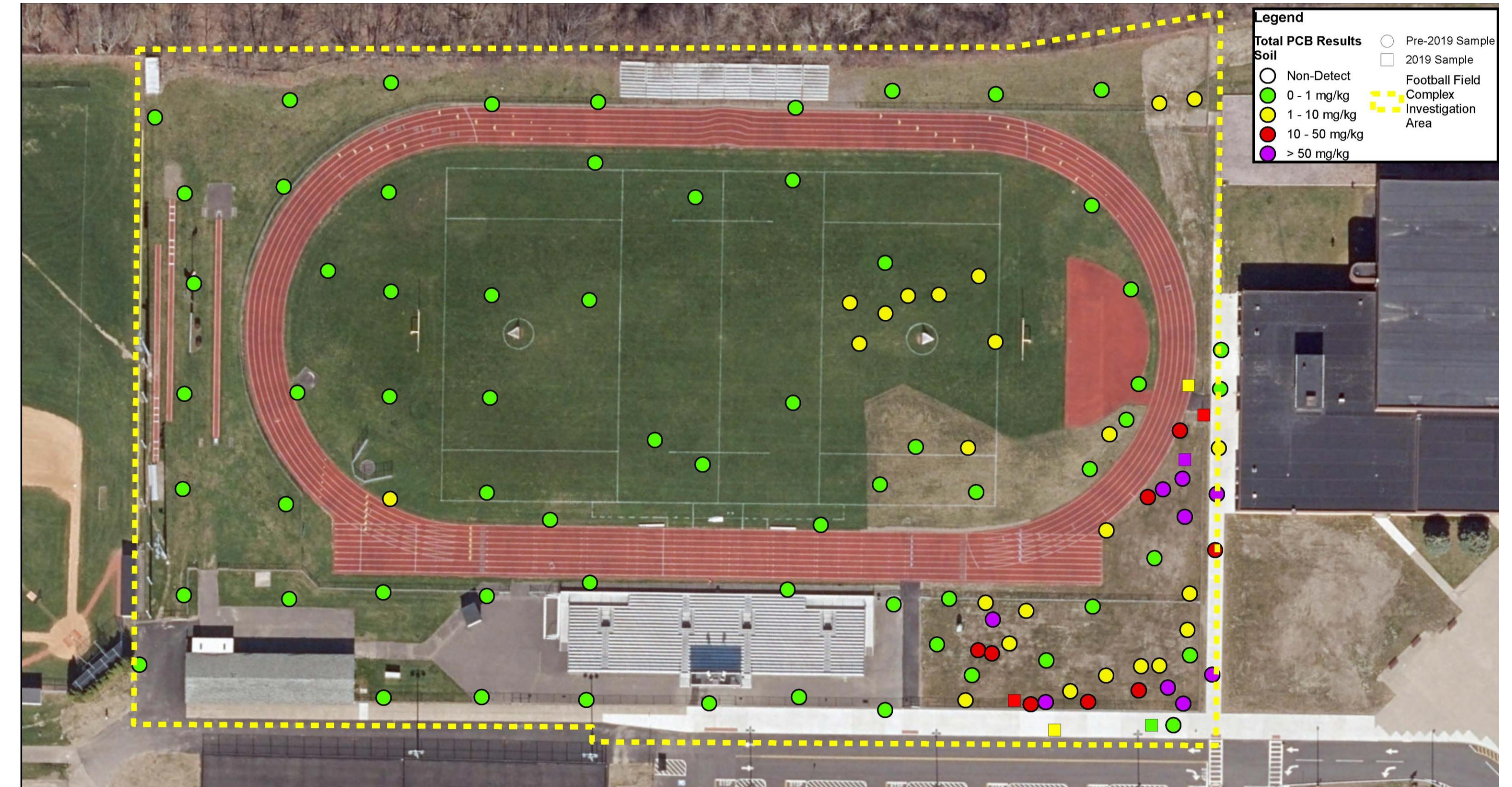
PCBs in Subsurface Soil: 8 to 10 feet below ground surface
