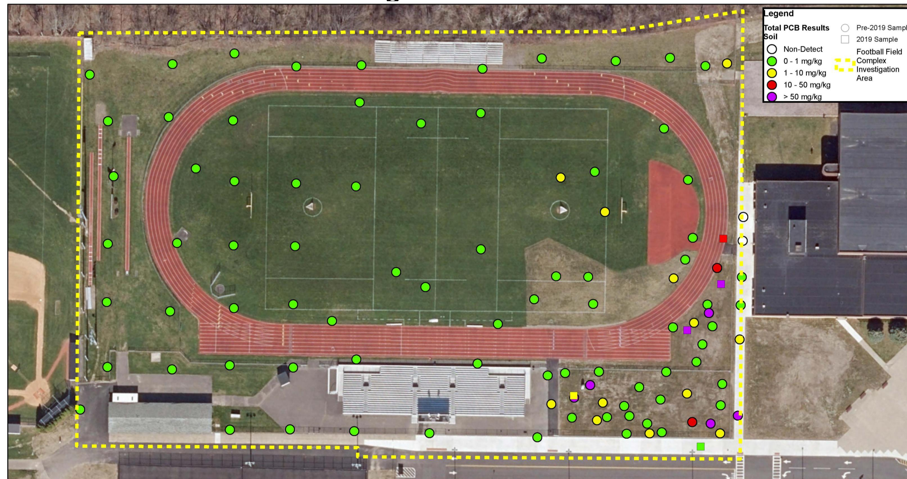
PCBs in Subsurface Soil: 10 to 12 feet below ground surface
