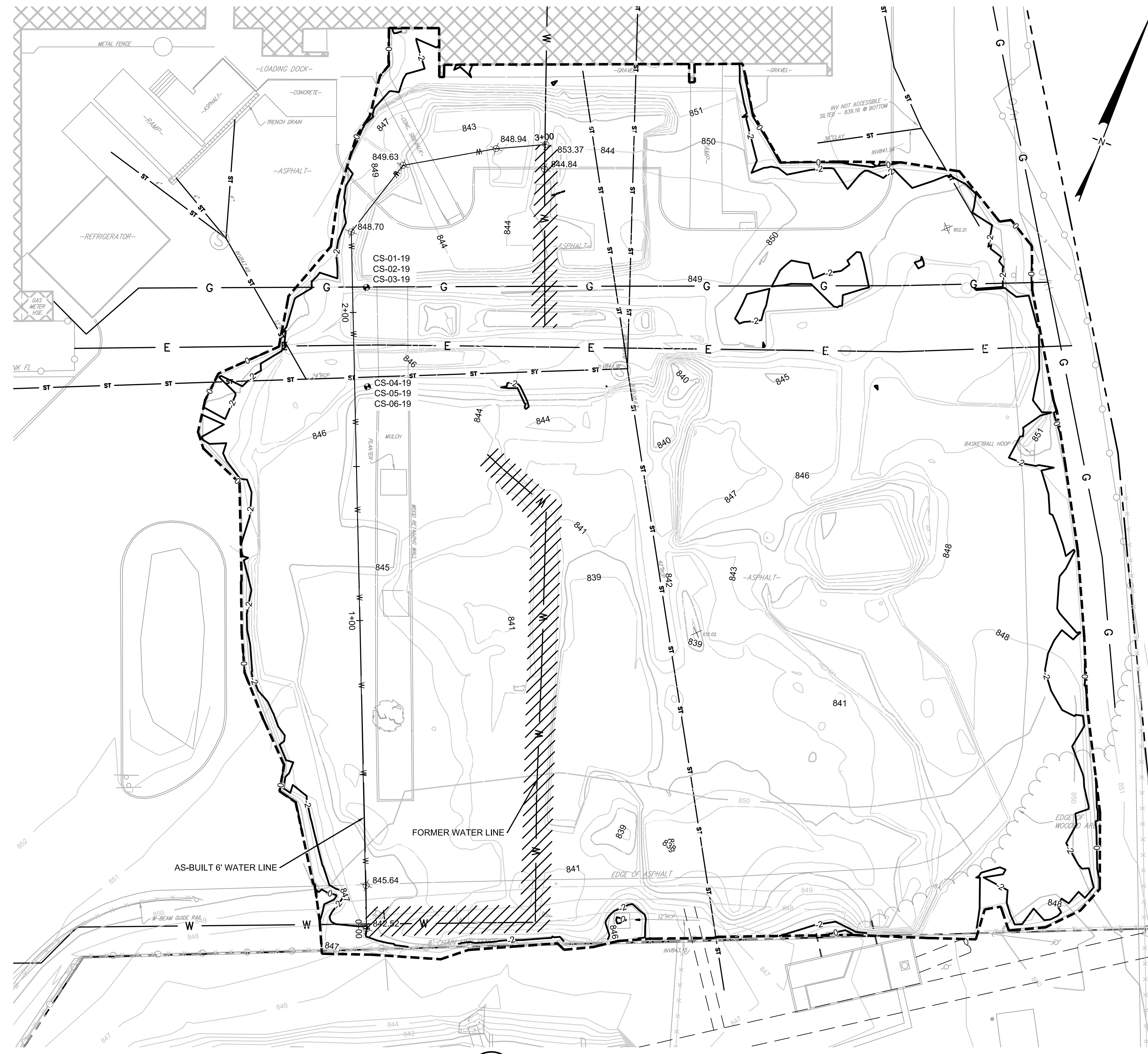
12 PLAN AS-BUILT WATER LINE RELOCATION SCALE: 1" = 20'
