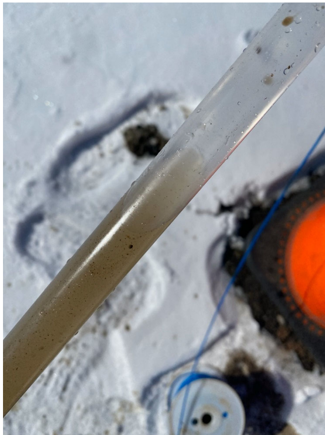
Photograph 2: Product in water in bailer at SB-3.
