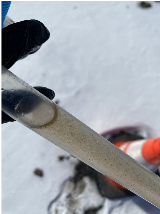
Photograph 1: Product in water in bailer at SB-1.
