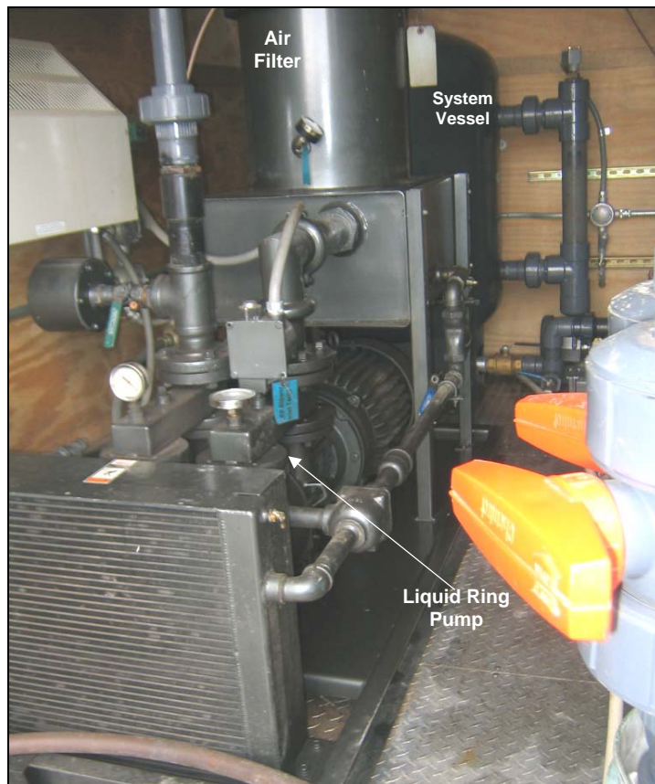
PHOTO 14 Detail of liquid ring pump, air filter and system vessel.
