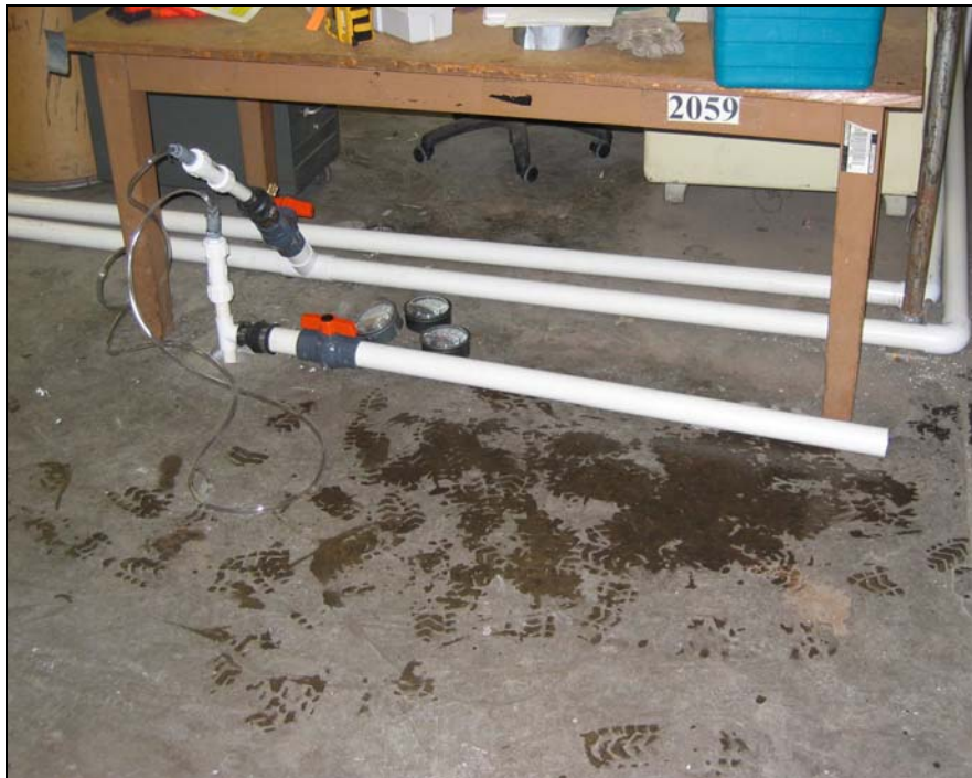
PHOTO 11 View of connection at MW105 operating in total fluids recovery mode. The length of PVC pipe visible to the right of the lower valve and the Magnahelic gauges behind the well are used for air flow measurement.
