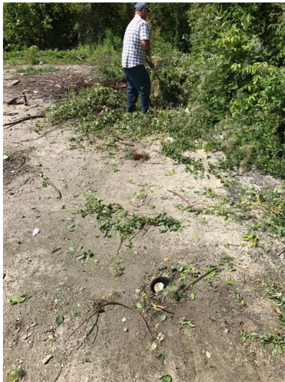
Monitoring well MW-12 with damaged curb box and missing j-plug (8-16-2017)
