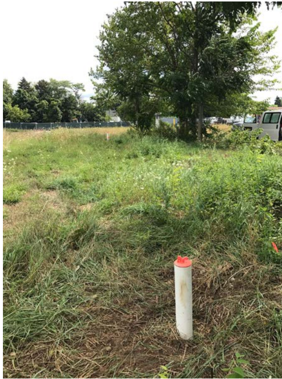
Well MWIRM-3 with repaired PVC stick-up and J-plug (8-31-2017)
