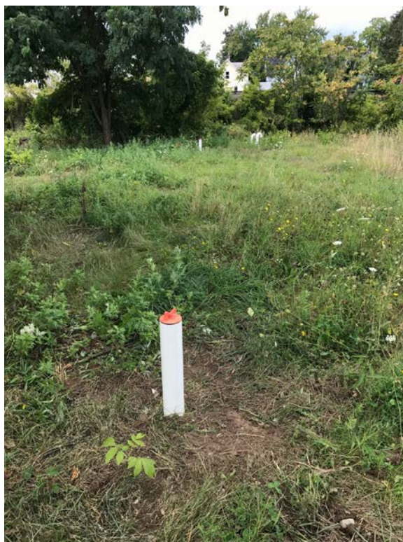
Well MWIRM-1 with repaired PVC stick-up and J-plug (8-31-2017)
