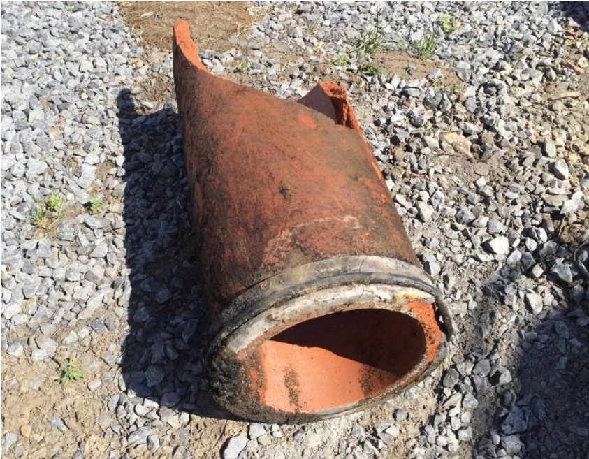
Discovered 6" pipe within 10" pip leading to sewer line
