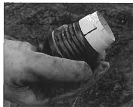
Figure 4.1. The spacer ring fits securely onto the MC5 Cutting Shoe.
