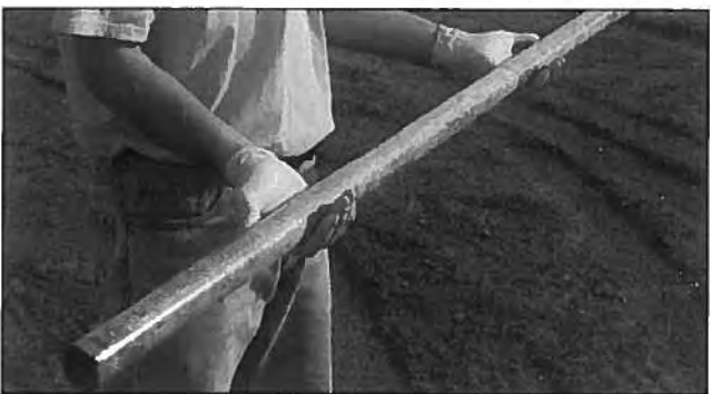
Figure 4.31. MC5 Liner filled with soil core.
