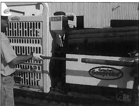
Figure 4.23. The MC5 Plug and a 1.25-inch light-weight center rod are inserted into the sample tube.
