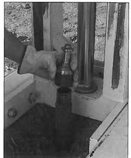
Figure 4.26. The pull cap is one way to remove the sampler from the ground.
