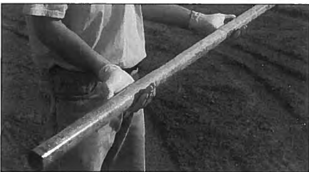
Figure 4.31. MC5 Liner filled with soil core.
