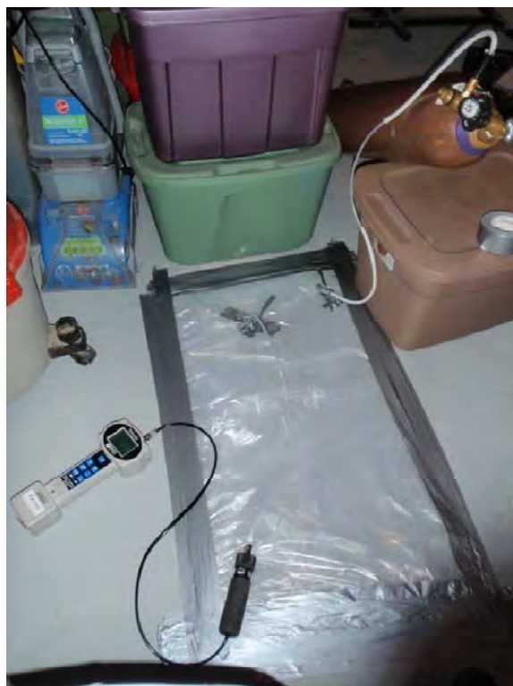
Conducting helium leak testing at Structure 08.
