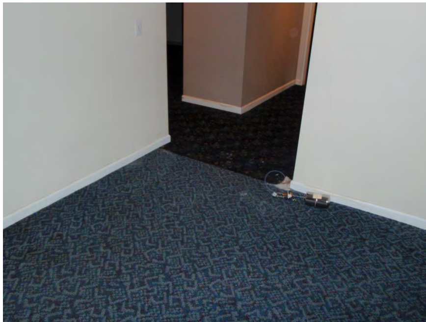
Sampling sub-slab soil vapor at Structure 06.
