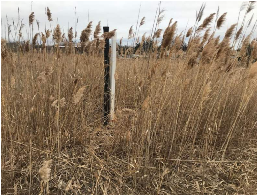
Photo 4c. Nested pair of risers/monitoring well for the product monitoring trench on site.
