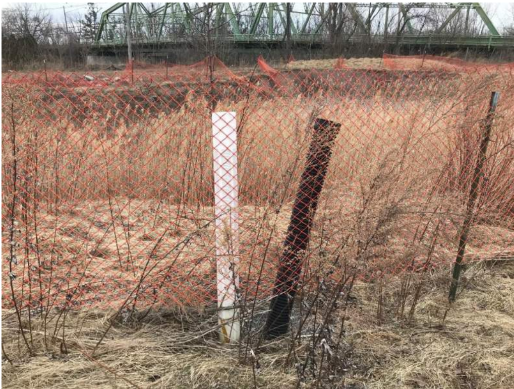
Photo 4a. Nested pair of risers/monitoring well for the product monitoring trench on site.
