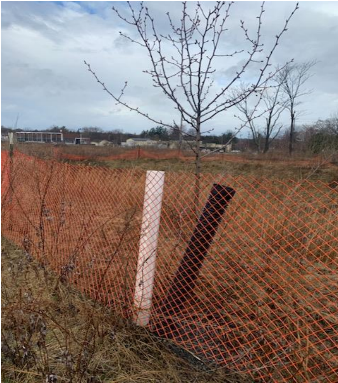
Photo 3. Nested pair of risers/monitoring well for the product monitoring trench on site.
