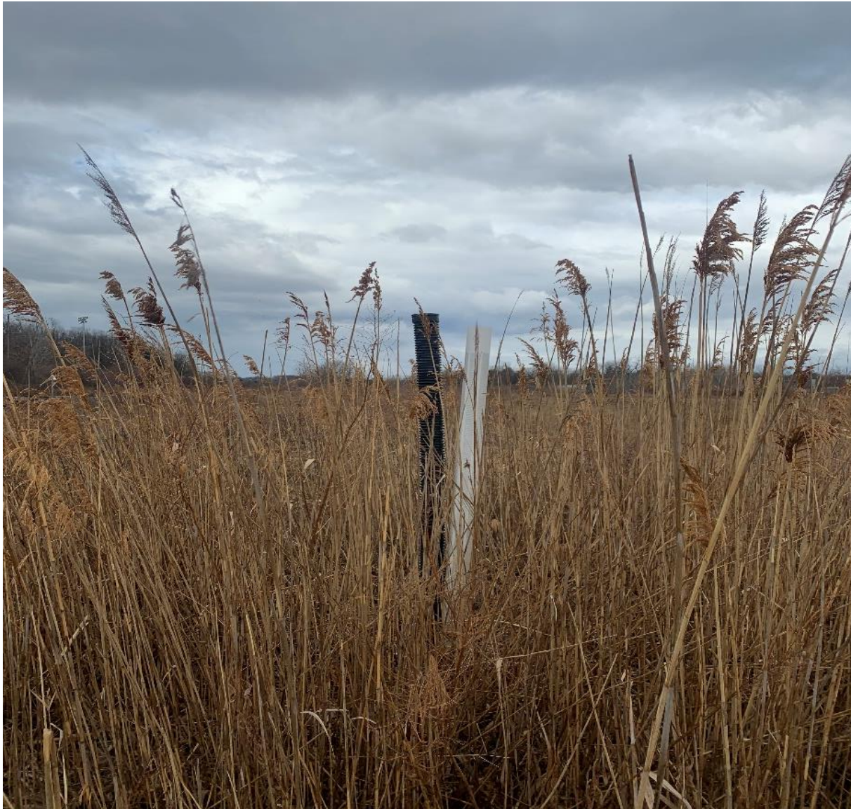
Photo 3c. Nested pair of risers/monitoring well for the product monitoring trench on site.
