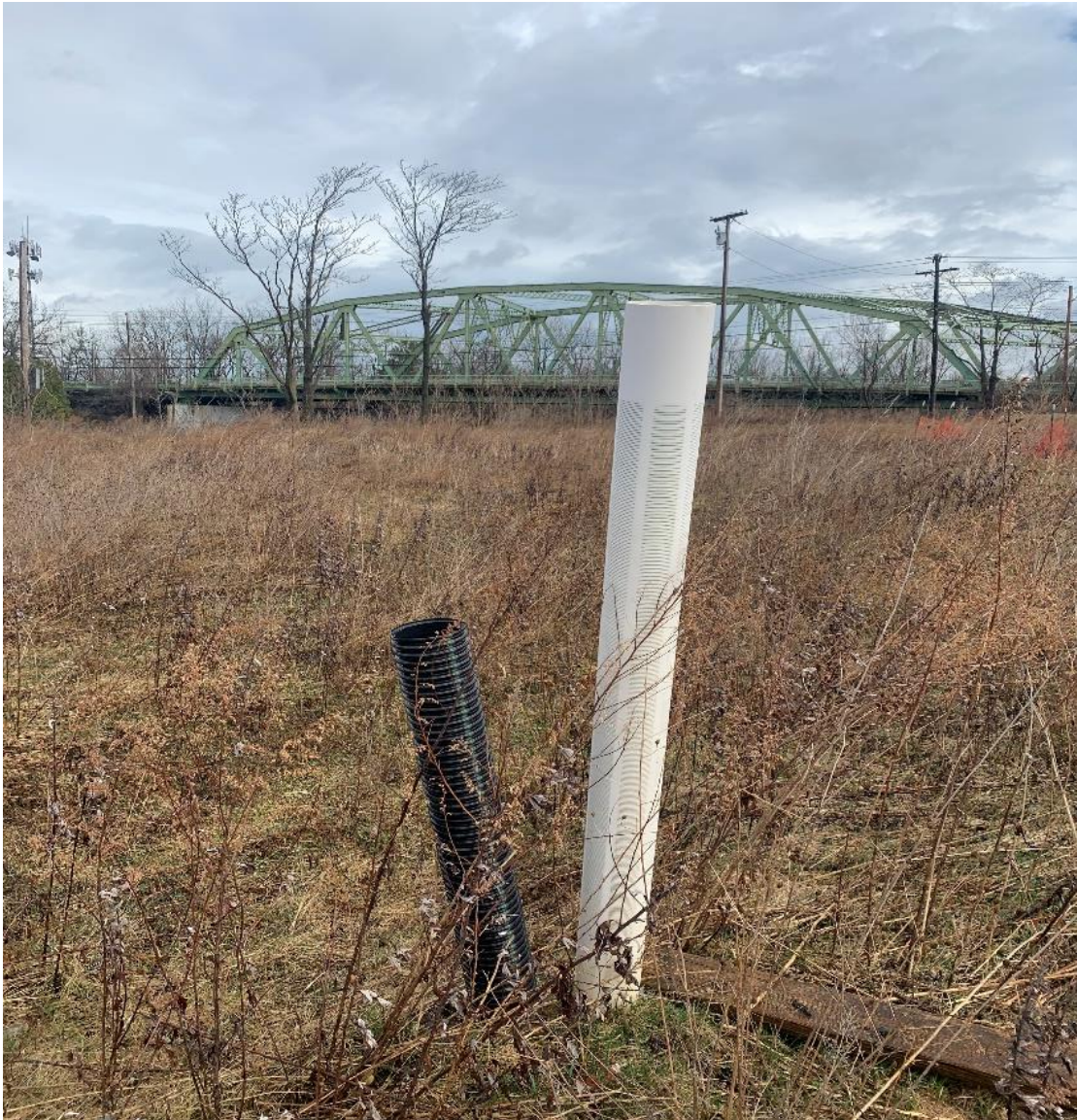
Photo 3b. Nested pair of risers/monitoring well for the product monitoring trench on site.
