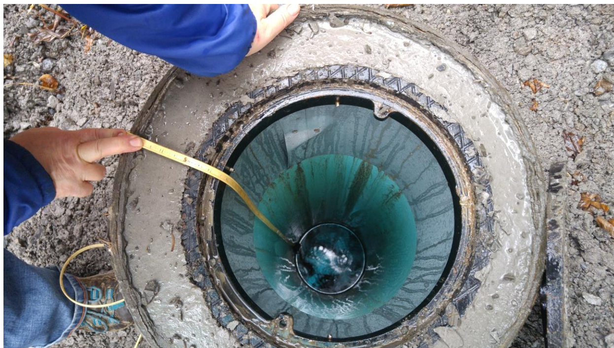
Measuring LNAPL accumulation
