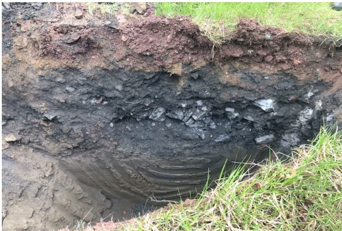
TP21-39 landfilled fill soils over lacustrine native soils
