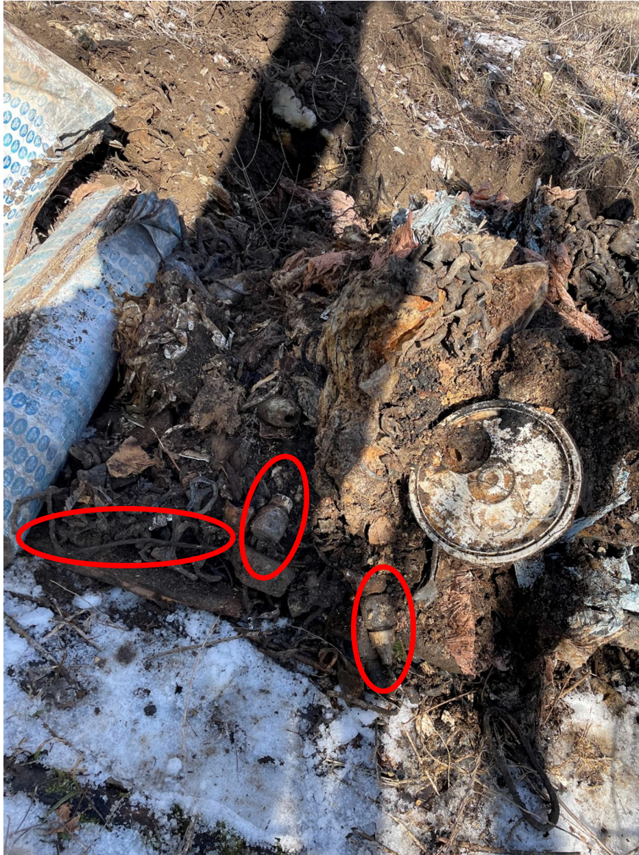
Photograph No. 3: Observed medical waste at Test Pit #3 (March 03, 2023). Note: Observed baby bottles and medical type tubing circled in red.
