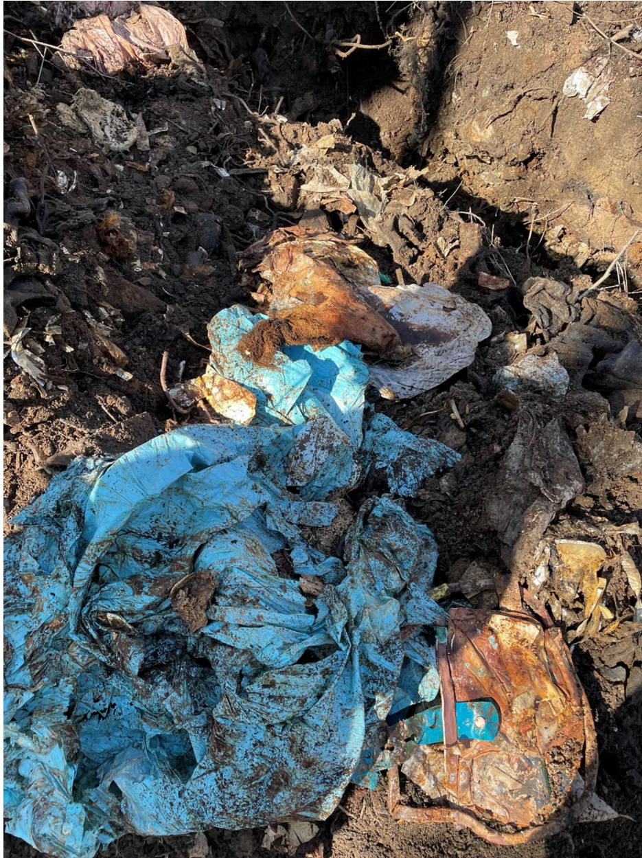
Photograph No. 2: Observed medical waste at Test Pit #3 (March 03, 2023). Note: what appears to be blue linens/medical waste bag, bedding or gauze material, tubing and IV bag.
