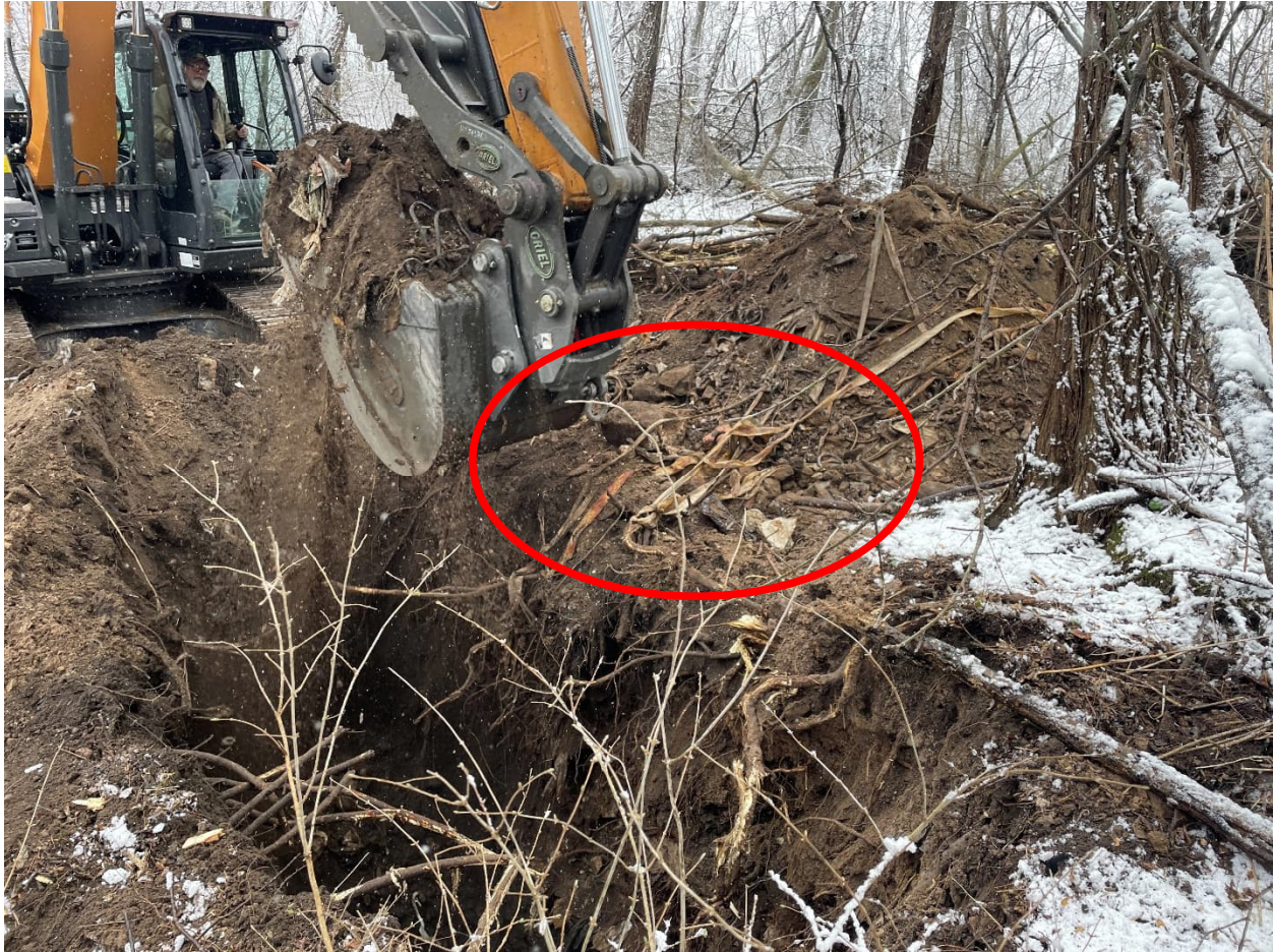
Photograph No. 5: Observed medical waste in Test Pit GEO-TP-04 (January 29, 2024). Note: Observed what appears to be several feet of stained gauze or bandage wrappings.
