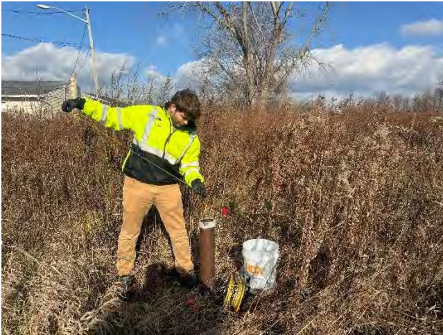
Photo No. 7 Purging of groundwater at OW-5.
