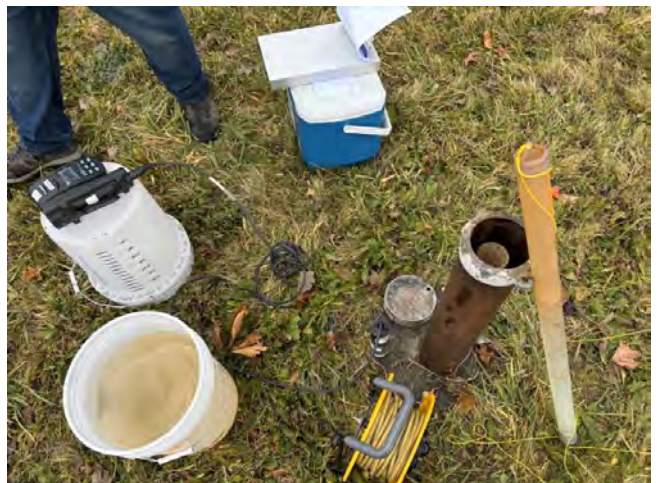
Photo No. 6 Slightly turbid groundwater found at OW-3.
