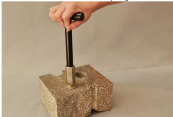
Figure 7. Removing the VAPOR PIN®
