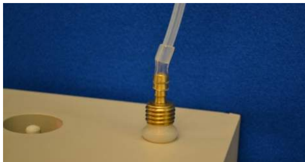
Figure 5. VAPOR PIN® sample connection
