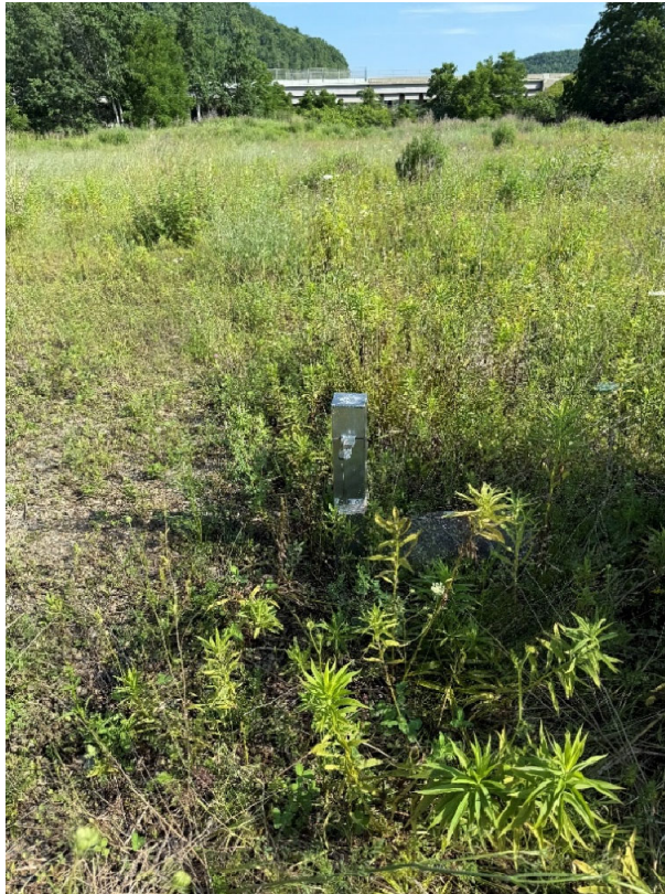
Typical view of a stickup monitoring well casing (foreground, i.e., MW-B) and vegetated soil cover (background) located on the central portion of the Site, facing north.
