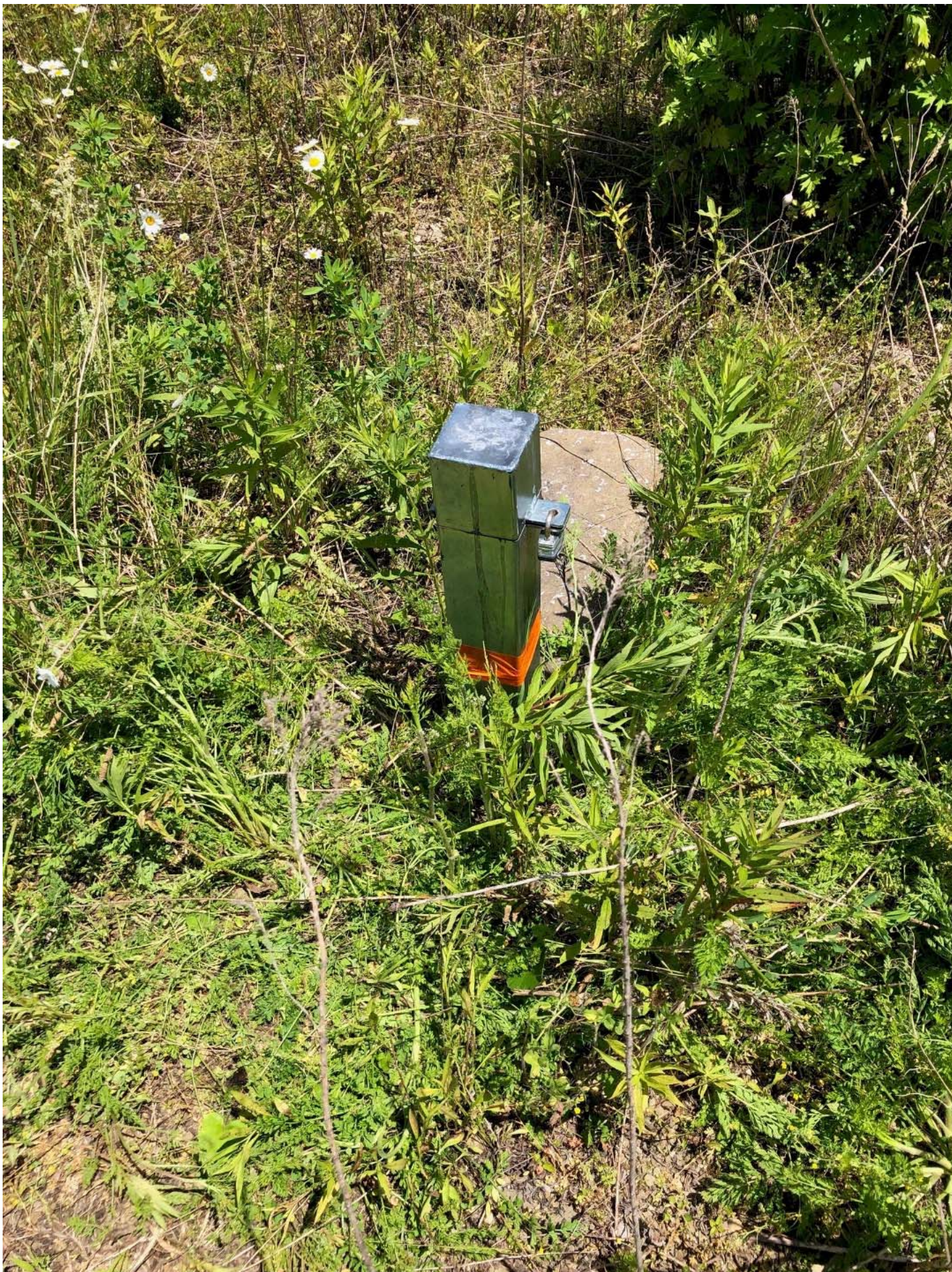
View of the protective casing for monitoring well MW-B, located on the central portion of the Site.
