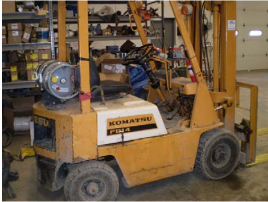
Propane operated fork lift within warehouse of Site building
