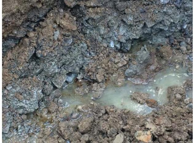
Photo 5: LNAPL and petroleum-impacted soils encountered at TT-3.
