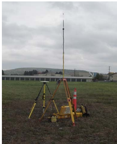
Trimble 5700 Global Positioning System base station
