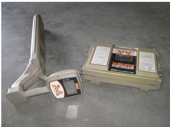
Subsite 970 utility locator
