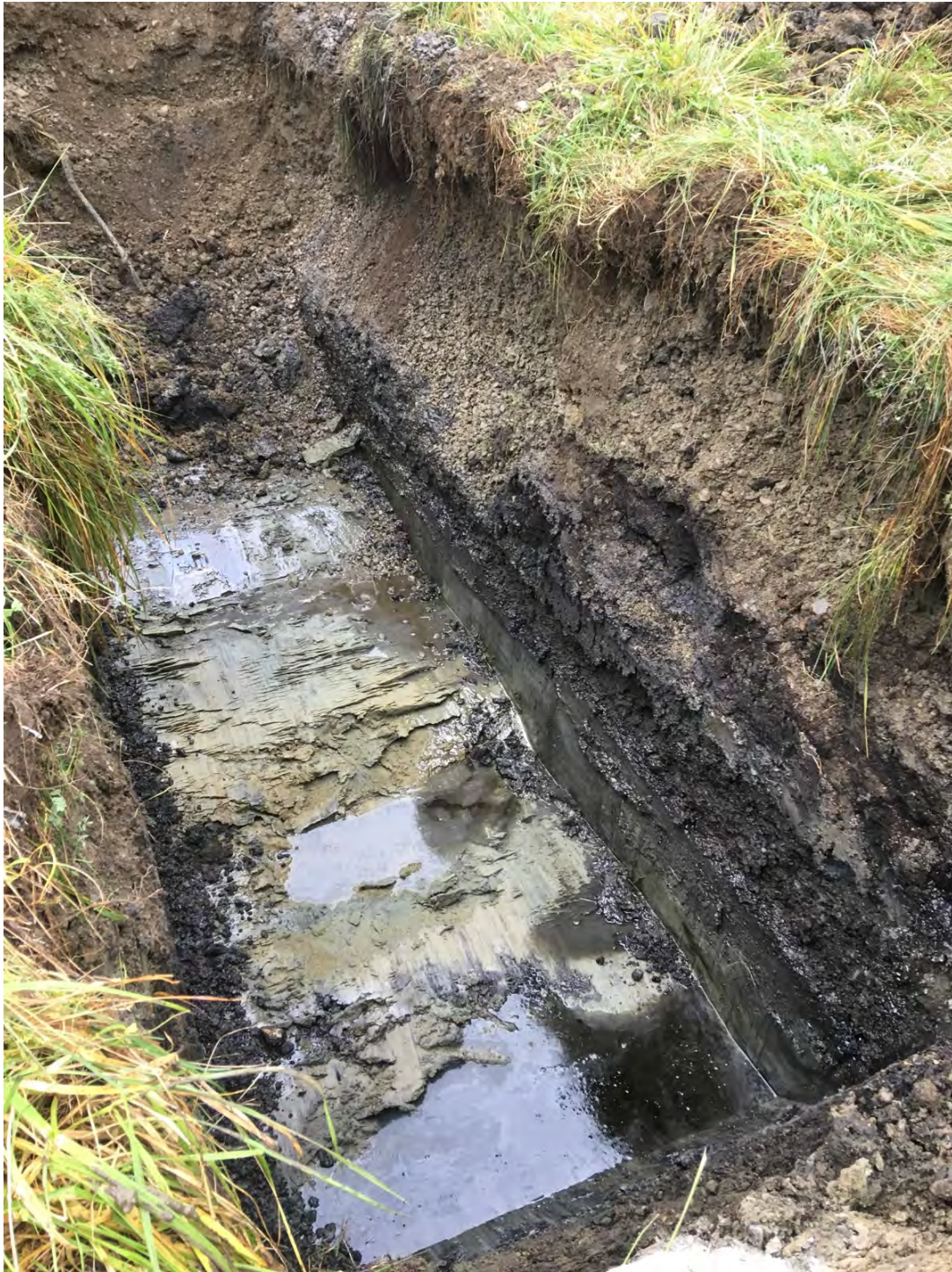
Photo 1: TP 187 - Suspected GCM encountered from 4-10 ft bgs; Confining clay layer encountered at 10 ft bgs.
