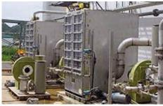
**Pre-treating** sing ir Strippers Two pharmaceutical plants in Puerto Rico use large SBR systems to treat wastewater. New regulations require them to treat the SBR off-gas. Instead of installing a very large CATOX, they decided to pre-treat the wastewater with a more efficient E-Z Tray Air Stripper before it enters the SBRs so they can use a much smaller CATOX unit.
