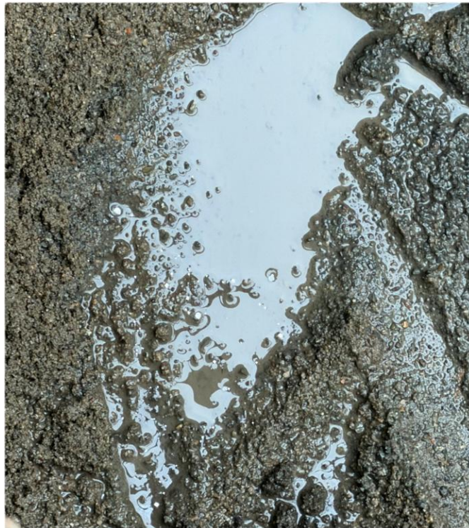
Photograph 2: An up-close view of the suspect elemental mercury beads within the sediment of the valve pit.
