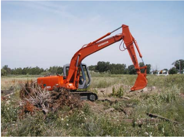
The HITACHI EX 120 moves a brush pile out of the way to begin excavating Area D
