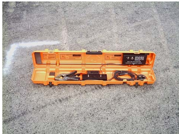
The instrument used is a Schonstedt MAC – 51 Bx
