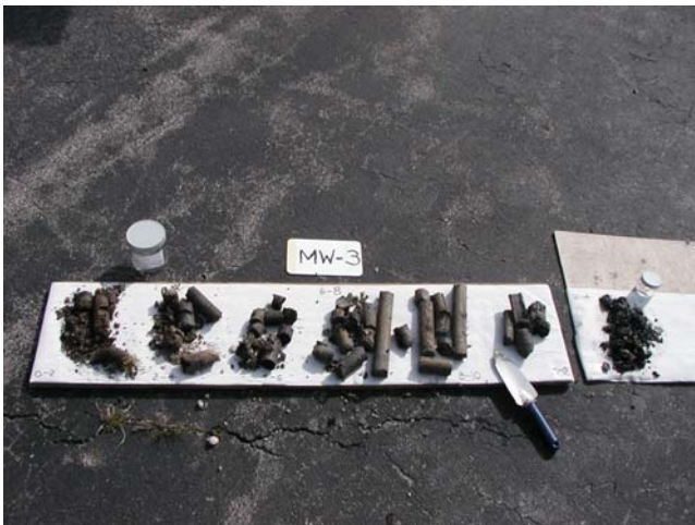
Soil borings from MW-3 laid out in two foot increments
