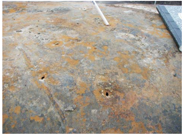
Holes were corroded right through UST-1
