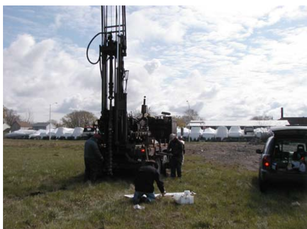
IEG field technician collects soil samples and tests for VOCs while SJB crew drills
