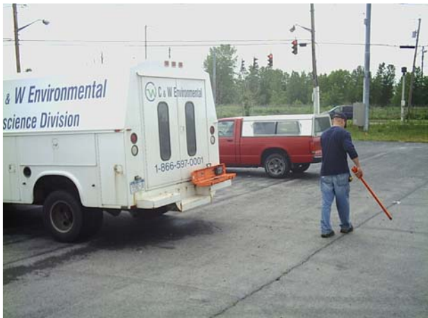
C & W crew uses metal detector to search for USTs
