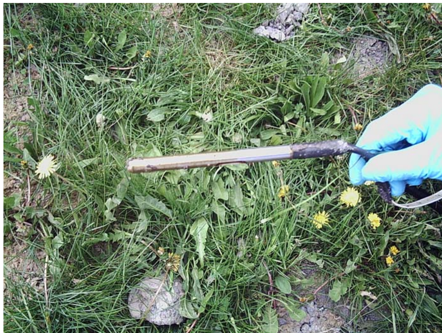
Product on tip of Water Level Meter at Piezometer TPMW 10
