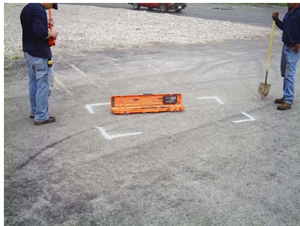
The strongest reading gets a further inductive test
