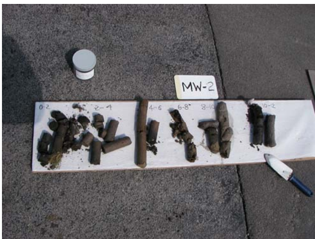
Soil borings from MW-2 laid out in two foot increments
