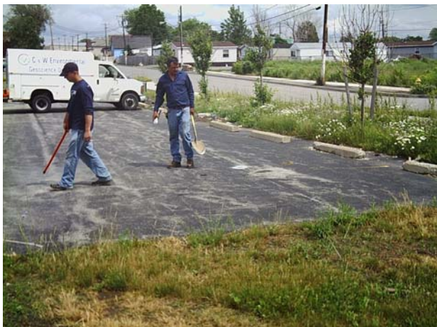
Readings over asphalt are marked with white paint
